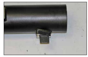
16. Install the mass air sensor into the K&N® intake tube and secure with the provided hardware.
