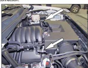
3. Disconnect the two crank case vent tubes from the intake plenum.
