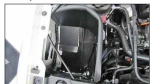
9. Install the heat shield assembly and secure to the air box mounting plate location using the three factory bolts from step #7.
