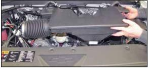
5. Remove the intake plenum from the vehicle.
