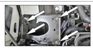
7. Remove the four bolts securing the air box mounting tray and then remove the tray from the vehicle.
