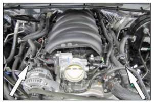
12. Remove the two factory crank case vent tubes from the vehicle.
