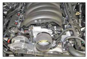
13. Install the provided coupling hose (08698 for 5.3L, 08497 for 6.2L) onto the throttle body and secure with the provided hose clamps.
