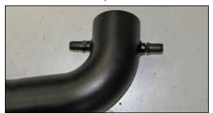
17. Install the two provided crank case vent fittings into the K&N® intake tube as shown.
