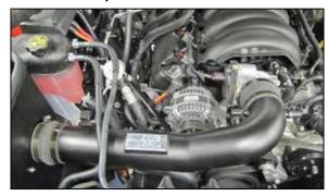
18. Install the K&N® intake tube into the hose at the filter adapter and then into the hose at the throttle body. Adjust the tube for proper fit and then secure with the provided hose clamps.
