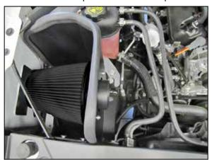
11. Install the filter assembly into the heat shield filter top first, then rotate the filter and pass the adapter through the hole in the heat shield. Secure the filter adapter to the heat shield using the provided hardware.
