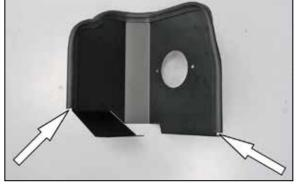
8. Install the provided edge trim onto the heat shield as shown.
